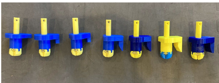
Iterations of our grabber (left to right - oldest to newest)
