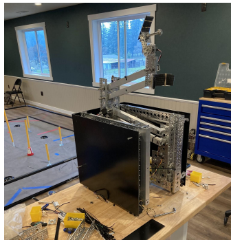
Our original Aluminum/PE composite encasement
